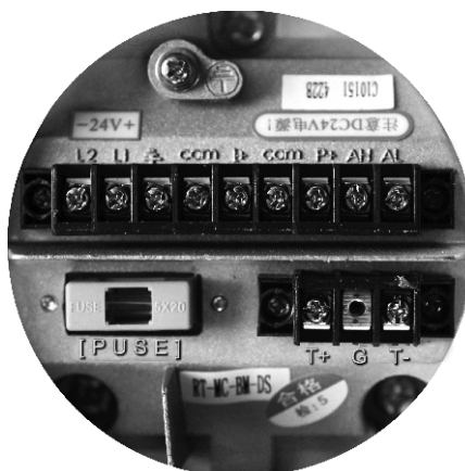
Fig. 6.3.4 Wiring terminal diagram of circular meter
